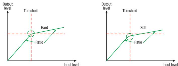
“Method”: this activation method defines how the transition between compression and non-compression should be done. The “Soft Knee” setting is recommended for instrumental sound, “Hard Knee” for voices (suppressing “pop” sounds in talking and singing).
