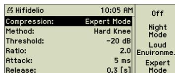
The dynamics compressor limits the range of dynamics of the audio material. When the defined threshold level is reached, the compressor compresses the signal according to a certain ratio. Attack time and release time define how fast the compression begins and ends.
