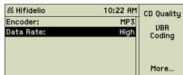
“Date Rate”: here you choose the MP3 quality level which the imported song should be encoded to. The Hifidelio has a data rate level called “CD Quality” which is equivalent to 320 kbit/s. Additionally, the MP3 format files can be encoded using Variable Bite Rate (VBR). If the VBR encoding is enabled, you can then set its quality level.
