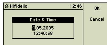
Adjust date and time with the help of the Turn&Select wheel (11) (see section 6.1.4 «Date & Time» on page 27) and press the function key
