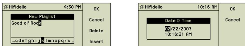
With the help of the inner Select wheel (11), select a character from the alphanumerical list at the bottom and confirm your choice by turning the outer Turn ring (11) slightly to the right. Function keys  $F_3$  “Delete” and  $F_4$  “Insert” help correcting typos. When finished, press the function key  $F_1$  “OK”.
