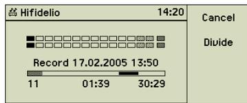
The recording is stopped automatically when the maximum recording time is expired or after the preset time of silence (see section 6.2.3 «Analogue Recording» on page 29). You may end it manually by pressing the Stop button (4 **(■)**). Pressing the Stop button (4 **(■)**) stops the paused recording.
