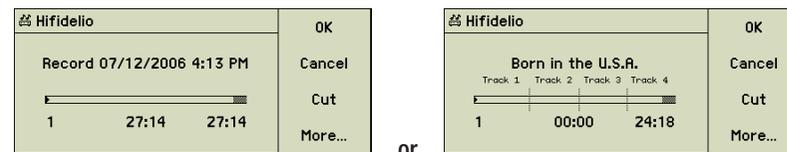
The bar shows a section of about 15 minutes of the recording. Depending on the position of the cursor, the remaining parts are displayed as grey-hatched elements at the left or the right end of the bar.
