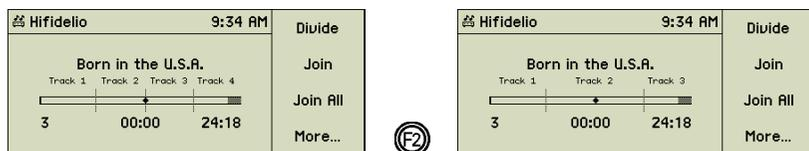
If the cursor is inside a track, press the function key
