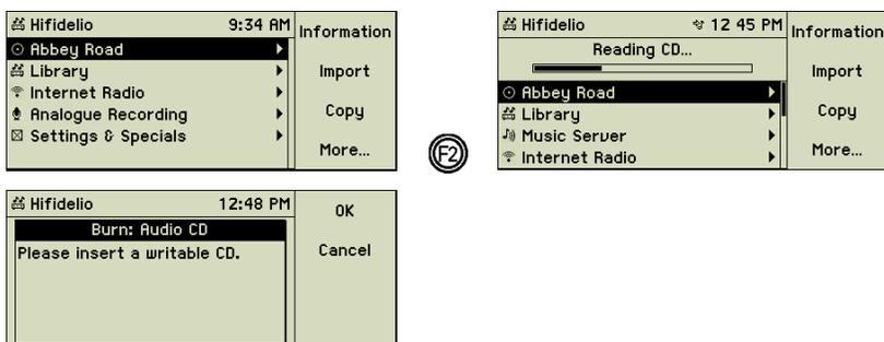
The Hifidelio reads all tracks of the audio CD and then asks you to insert a fresh CD-R into the CD slot (2). Remove the ejected audio CD and insert a CD-R into the CD slot (2). The burning process starts automatically.
