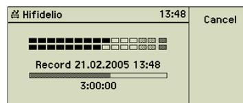
Manually adjusted record levels are never ever changed by the Hifidelio, even if this yields to an over modulation of the recording.
