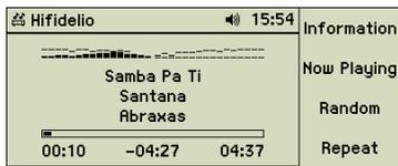
“Spectrogram”: toggles the display of banded frequency levels during the playback of songs.
