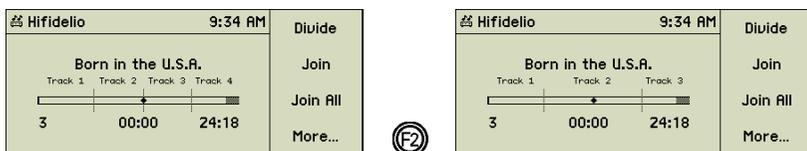
If the cursor is inside a track, press the function key
