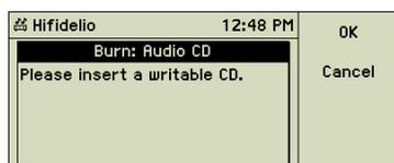
A message on the Hifidelio's display asks you to insert a fresh CD-R into the CD slot (2). The burning process begins automatically and proceeds according to your settings (see section 6.2.4 «CD Burning» on page 29). After completion of the burning process, the newly burned CD is automatically ejected.
