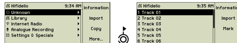
If the inserted music disc is a data disc (CD or DVD), the disc name is displayed at the top of the main menu. In the case of existing folder structure on the disc, the submenu first shows the list of the artists and then their albums and songs. A data disc contains songs with different audio formats (MP3, FLAC, AIFF etc.). If these formats support meta tag information, the names of the artists, albums and songs are shown on the display.
