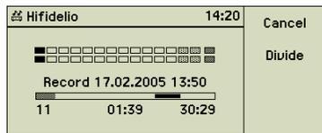
The recording is stopped automatically when the maximum recording time is expired or after the preset time of silence (see section 6.2.3 «Analogue Recording» on page 29). You may end it manually by pressing the Stop button (4 **(■)**). Pressing the Stop button (4 **(■)**) stops the paused recording.
