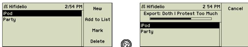
Select the MP3 player as the target playlist and press the function key **(F2)** “Add to List” to transfer the songs to the external player. The process of the import is shown on the display.
