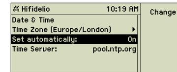
Select the menu option “Set automatically” and press the function key **F1** “Change”. A new option “Time Server” is displayed. You can change the preset time server by pressing the function key **F1** “Change” and then by selecting a server from the list.
