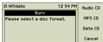
Choose the requested format. For an audio CD, the music files are first converted into an original audio format and then burned onto the CD. An MP3 CD only contains MP3 files (file names are limited to 64 characters); files with other formats are ignored during the burning process. A Data CD is the compilation of files regardless of their format (MP3, AIFF, FLAC, etc.).
